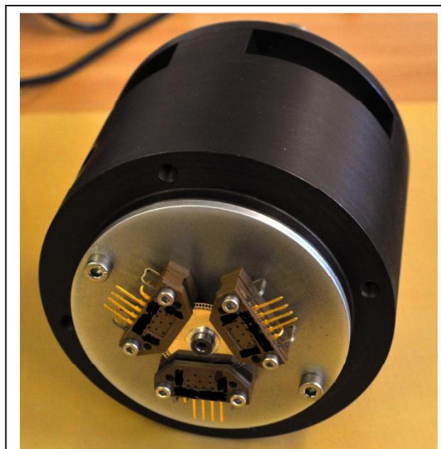
Figure 3. The commercial IME device, showing the encoder with three equally spaced optical read heads. The device has been designed with a standard attachment for testing machine tool bearings.
